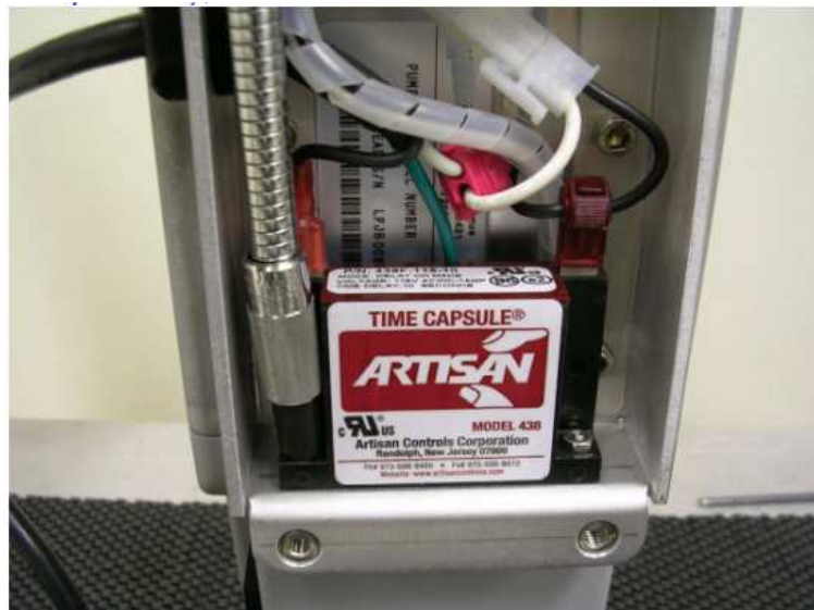
Figure 1-7 Timer Mounting and Harness Connection
