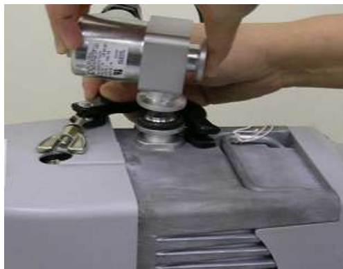
Figure 1-12 Installation of Inlet Valve with IDP Series Pump
